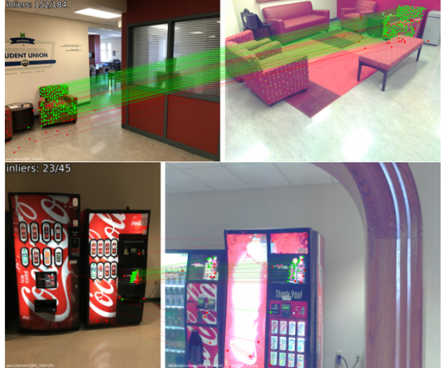
Figure 8. Failure cases on InLoc [70]. LightGlue sometimes matches repeated objects in the scene with strong texture, instead of the geometric structure.
