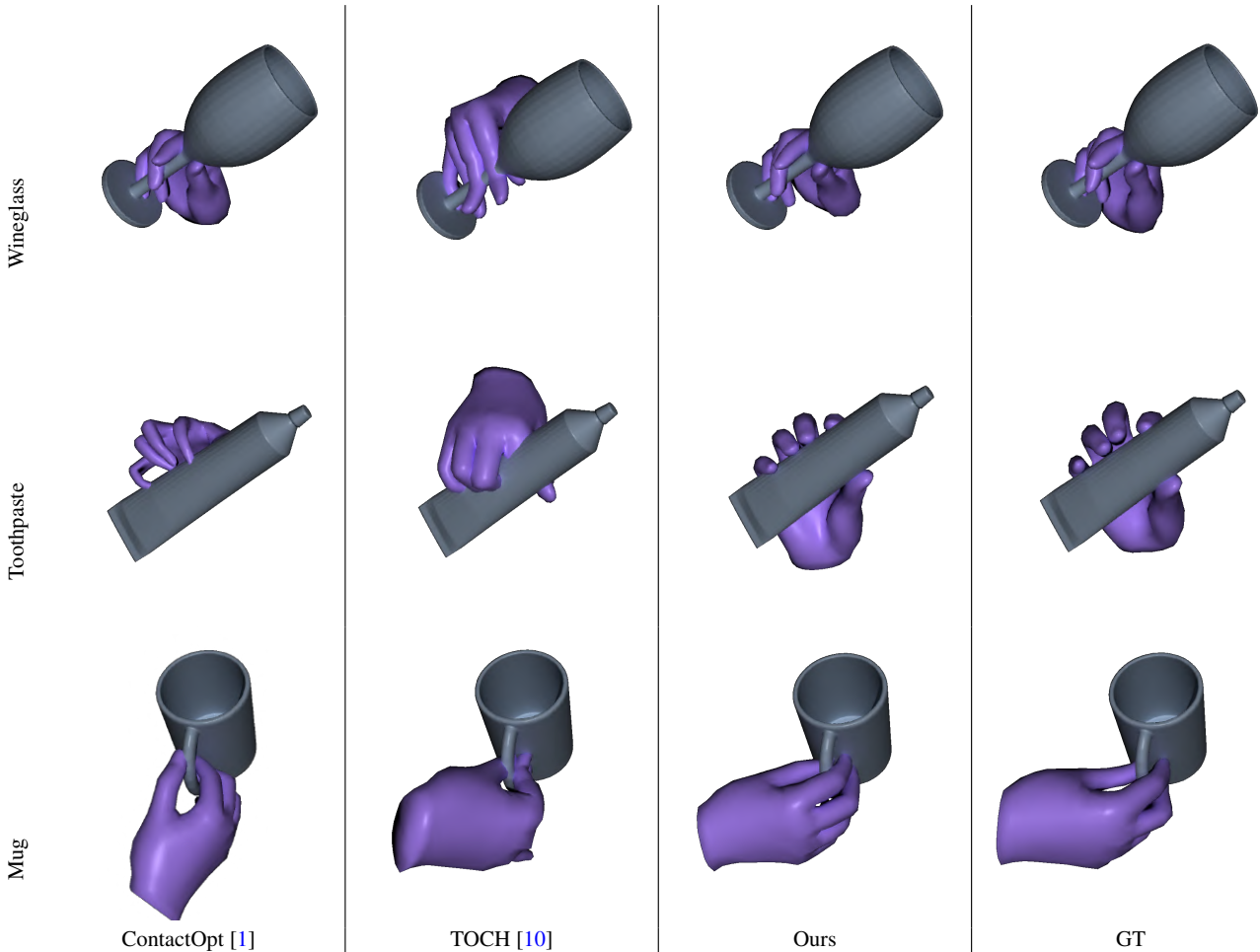
Figure 3: Contact Representation comparison against ContactOpt [1] and TOCH [10] on GRAB dataset [9]. Given the object and GT contact, we verify whether each method could recover the GT hand grasp. It can be seen both ContactOpt and TOCH exhibit failures in certain cases, whereas our method manages to achieve the closest reconstruction to the ground truth.
