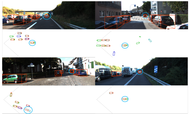
Figure 1: Qualitative results our MonoXiver with MonoCon [10] on KITTI validation set [3]. The ground truth is shown in green and blue. The prediction result is shown in red. We use top-1 prediction results for visualization.
