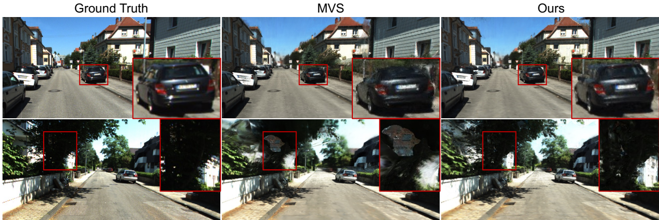
Figure S-2. Qualitative comparison of novel view synthesis on KITTI-360 dataset with neural rendering using meshes reconstructed from Multi-View Stereo (MVS). Cropped patches are scaled to highlight details. Reconstructed meshes from MVS are incomplete (e.g., the upper part of the car in the cropped patches in the first row) and contain occlusions (e.g., the building in the bottom-right corner of the cropped patches in the second row), leading to blurry and unreal rendering results.
