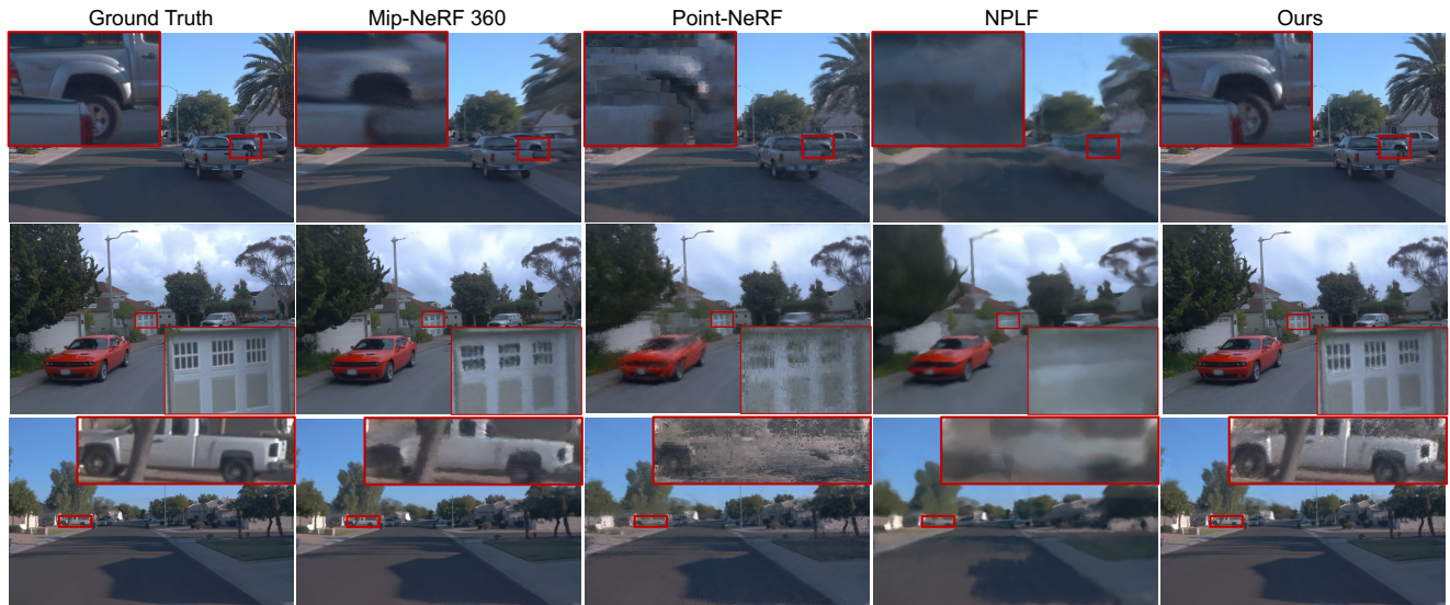
Figure S-7. Qualitative comparison of novel view synthesis on Waymo dataset. Cropped patches are scaled to highlight details. Due to the explicit and accurate surface modeling, the proposed method significantly outperforms baseline methods and can effectively recover texture details.
