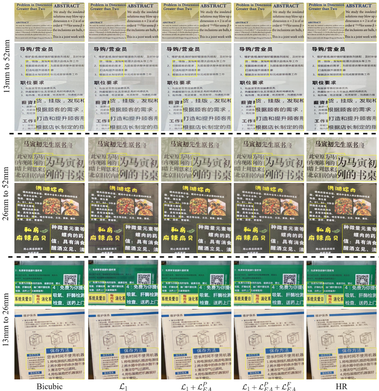
Figure 5. STISR results of ELAN models trained on Real-CE with different combination of losses. From top row to bottom row are results with zooming factors 4\times (13mm to 52mm) and 2\times (26mm to 52mm and 13mm to 26mm). From left column to right column are the results of bicubic interpolation, models trained with L_1 , L_1 + L_{EA}^P and L_1 + L_{EA}^P + L_{EA}^F and HR. Please zoom in for more details.
