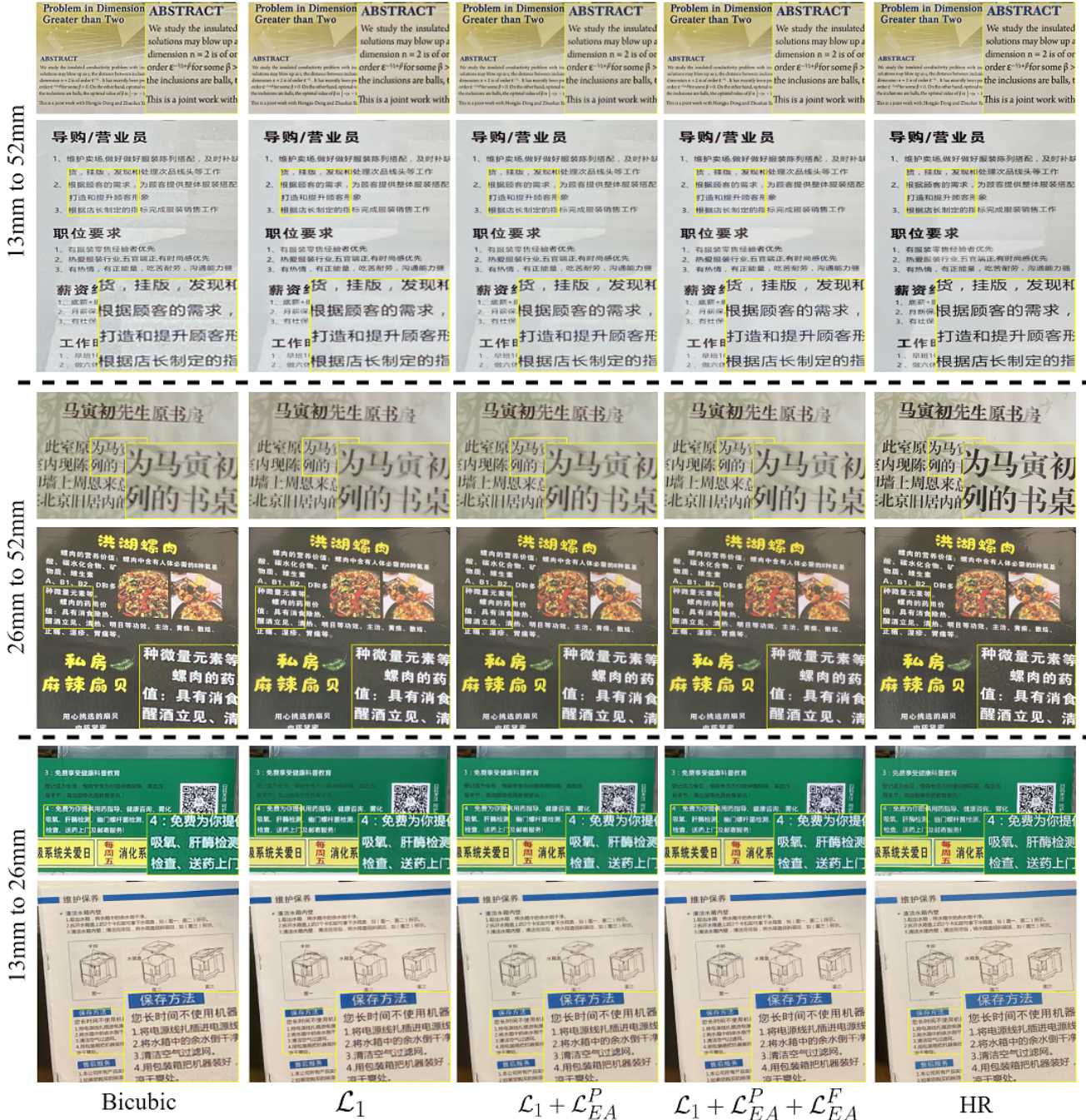
Figure 4. STISR results of RCAN models trained on Real-CE with different combination of losses. From top row to bottom row are results with zooming factors 4\times (13mm to 52mm) and 2\times (26mm to 52mm and 13mm to 26mm). From left column to right column are the results of bicubic interpolation, models trained with \mathcal{L}_1 , \mathcal{L}_1 + \mathcal{L}_{EA}^P and \mathcal{L}_1 + \mathcal{L}_{EA}^P + \mathcal{L}_{EA}^F and HR. Please zoom in for more details.
