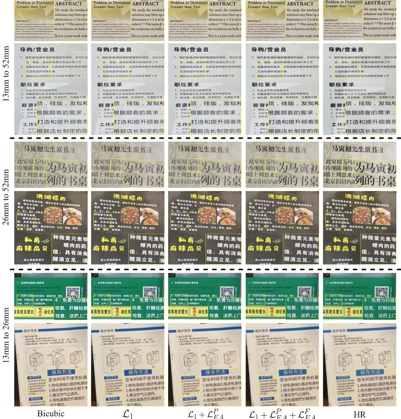
Figure 3. STISR results of RRDB models trained on Real-CE with different combination of losses. From top row to bottom row are results with zooming factors 4\times (13mm to 52mm) and 2\times (26mm to 52mm and 13mm to 26mm). From left column to right column are the results of bicubic interpolation, models trained with L_1 , L_1 + L_{EA}^P and L_1 + L_{EA}^P + L_{EA}^F and HR. Please zoom in for more details.
