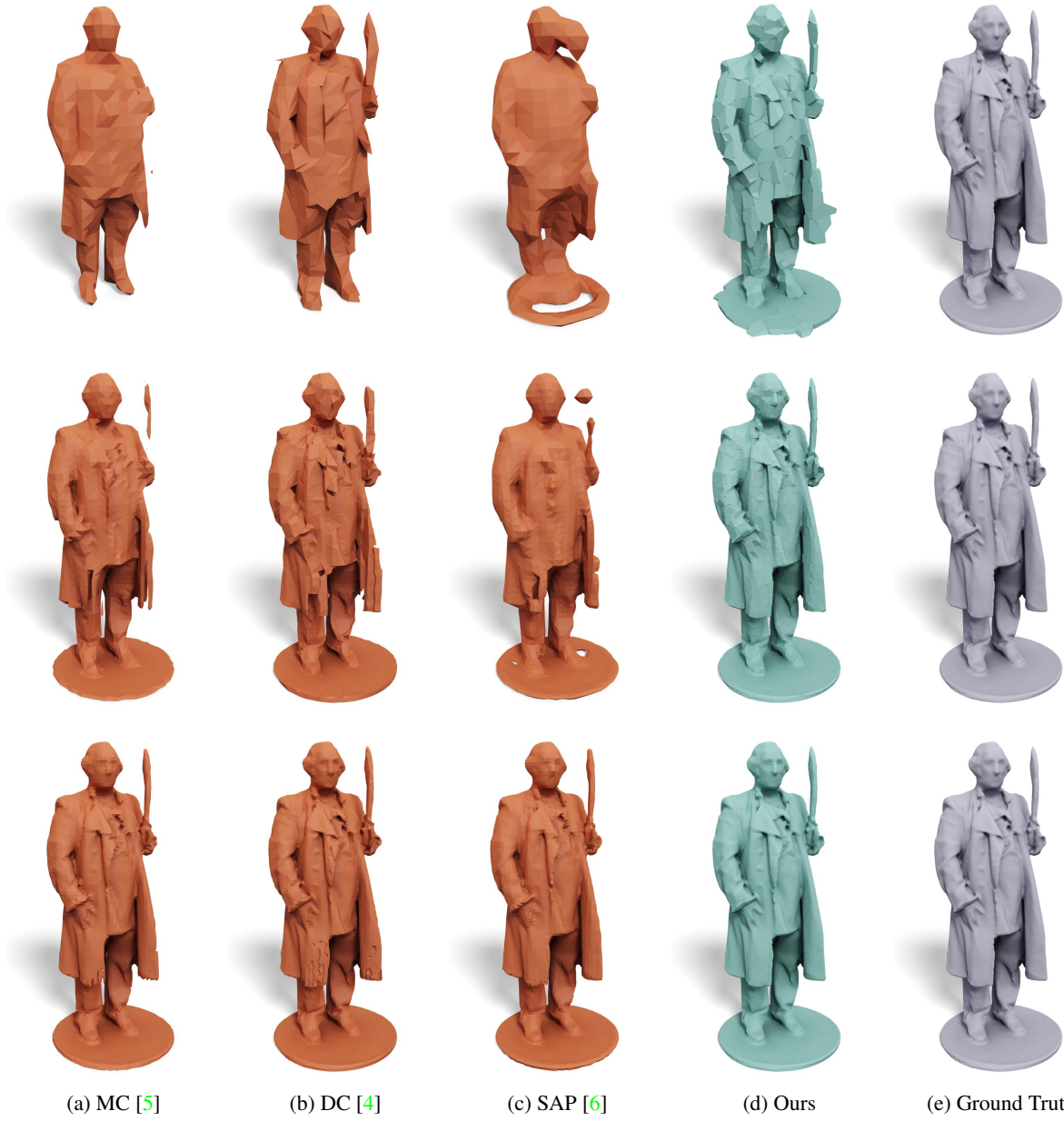
Figure 9: Visual comparison of optimization-based methods for grids of size 32^3 (top row), 64^3 (middle row), and 128^3 (bottom row)
