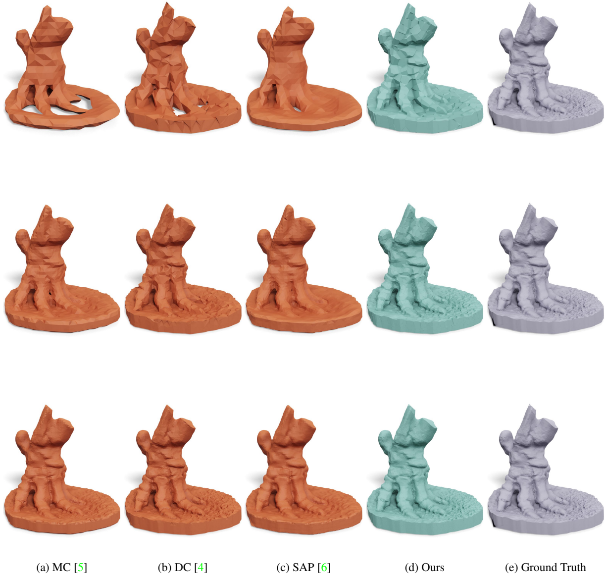
Figure 12: Visual comparison of optimization-based methods for grids of size 32^3 (top row), 64^3 (middle row), and 128^3 (bottom row)
