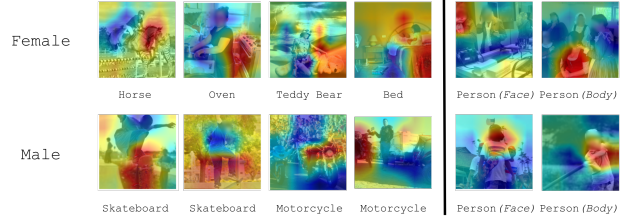
Figure 7. Visualizing model attention. On the left four images, the gender artifact model’s attention is on contextual objects and not the person, suggesting the model relies on spurious correlations to infer gender. On the right, the model’s attention is on the person. These qualitative CAM analyses suggest gender artifacts are embedded in the background of images (i.e., beyond the person) as observed by Hendricks et al. [31] and motivate future analysis in contextual objects.
