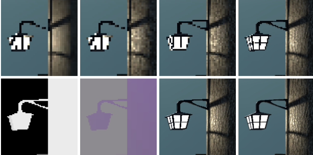
Figure 11. Example of data modalities available in the QRISP dataset. (first row, from left to right): Native 270p, Negative 2 mipmap biased 270p, Negative 1.58 mipmap biased 360p, Negative 1 mipmap biased 540p. (second row, from left to right): 540p depth, 540p motion vectors, Native 1080p, Enhanced 1080p
