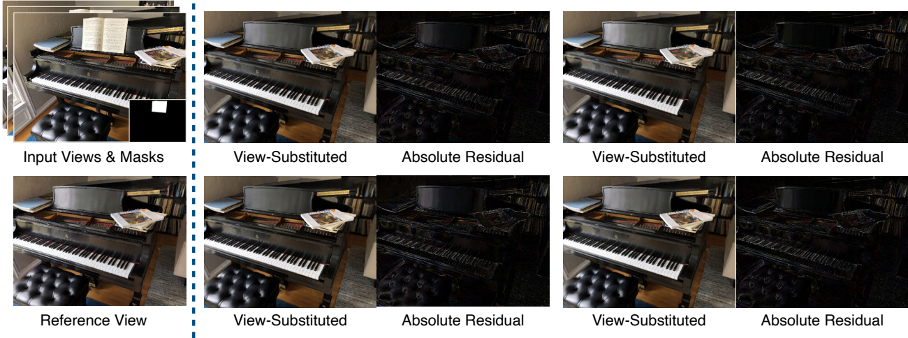
Figure 14: Overview of the outputs of our view-substitution method. The input views and masks (top-left) with their corresponding camera parameters, in addition to a single reference view (bottom-left), are the inputs to our multiview inpainting approach. On the right hand side, we show the view-substituted renderings, \{I_{r,t_1}, \dots, I_{r,t_4}\} , for four different target views, \{t_1, \dots, t_4\} . For each view-substituted image, I_{r,t} , we also provide the absolute value of the residual, |I_r - I_{r,t}| , to illustrate the view-dependent effects provided by our approach. Notice that all of the view-substituted images are looking at the scene from the reference camera, but the rendered colours are from different target cameras.
