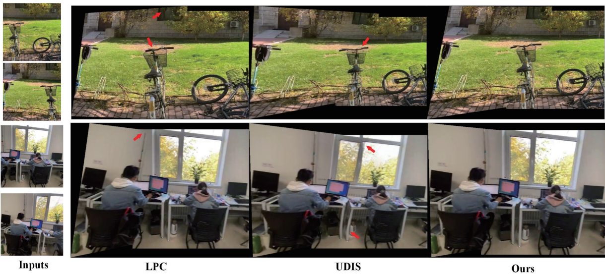
Figure 14: Comparative results of complete stitching frameworks. LPC[4] and UDIS[8] leverage perception-based seam cutting[6] and reconstruction[8] as the composition methods.
