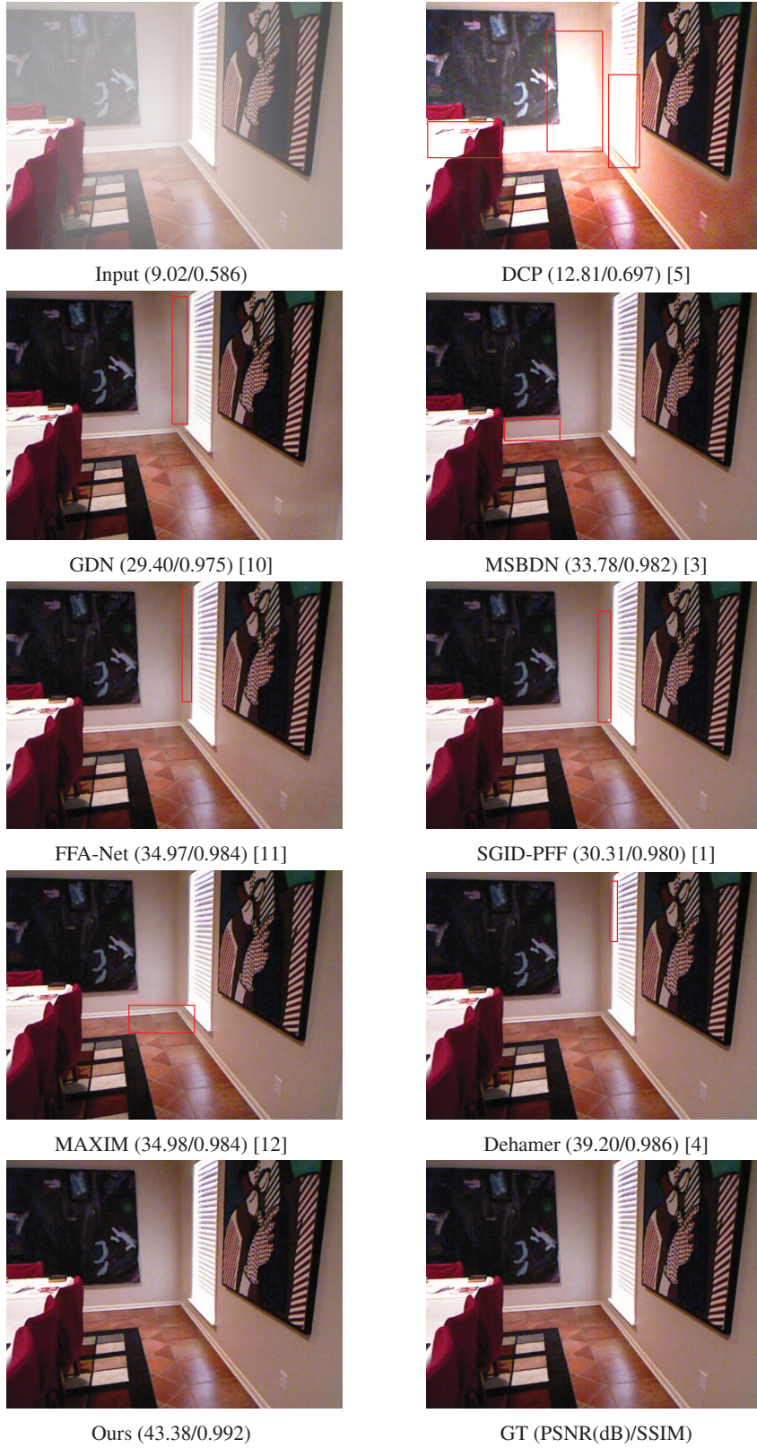
Figure 4: The qualitative comparison on SOTS-Indoor [8]. Our result has the best visual quality and details.
