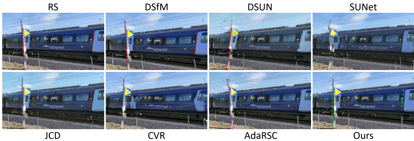
Figure 12: (a) Visual comparison against the state-of-the-art RSC methods in highly dynamic scenes of Train at speed video sequences. The camera was rotating rapidly to film the forwarding train. All existing RSC solutions fail in such a dynamic scene. In contrast, Our method corrects distortions properly.
