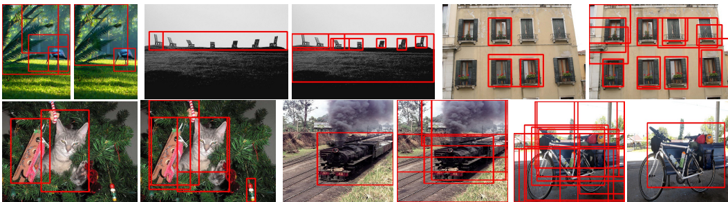
Figure 6: Effect of patch size: Each row illustrates three pairs of images showing results of MOST using ViT-S/16 (left) and ViT-S/8 backbones respectively. MOST with ViT-S/8 backbone can localize smaller objects but results in noisier outputs.
