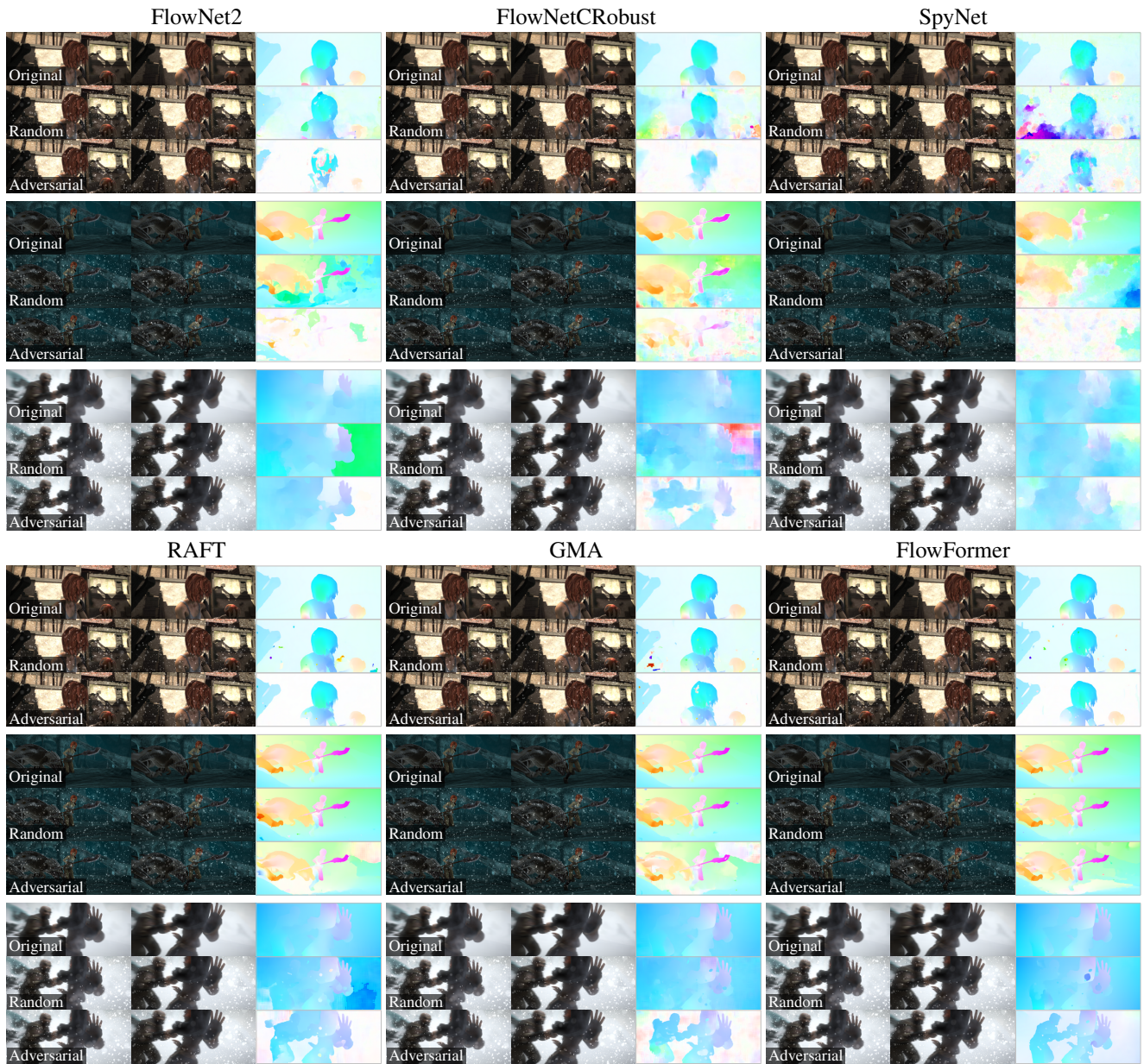
Figure A.3. Snow . Qualitative results for 3000 snowflakes on images from the Sintel final dataset with random initialization and adversarial optimization with optical flow predictions for FlowNet2 [3], FlowNetCRobust [9], SpyNet [6], RAFT [10], GMA [4] and FlowFormer [2], as extension to Main Fig. 6. See also Figs. A.4, A.5 and A.6.
