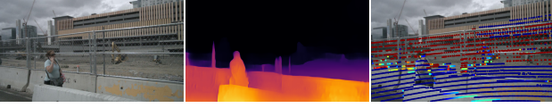
Figure 2. Illustration of thin structures. We depict an example frame, prediction, and error map from the NuScenes dataset. The fence in the picture poses a problem for our depth estimator since it is partially transparent. Further, since behind the fence, there is a large free space, we observe a large Sq. Rel. score for the areas that are predicted as background.
