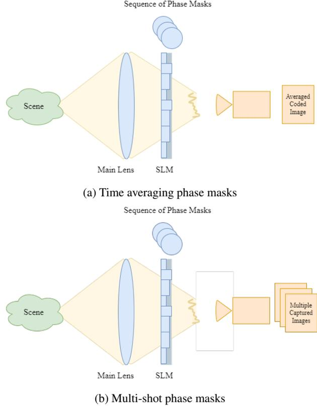
Figure 4: **Time averaging and multi-shot optical systems.** Observe that multi-shot systems capture multiple coded images, while time averaging only captures one. This means our system is more light and memory efficient.
