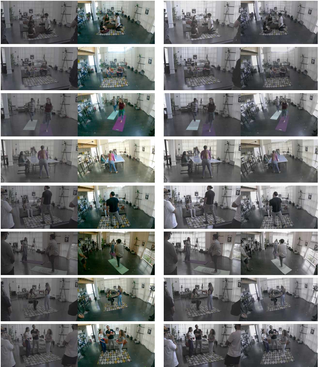
Figure 3. Color calibration. For 8 different scenes (rows), we show a pair of frames from a DSLR and a GoPro sensor before color equalisation (left) and after equalisation (right). Please note the discrepancy in colors on the left due to hardware differences. We equalise images by transforming them into a common sRGB color space and matching a color-checker target. Equalised colors enable combining sensors for training new-view synthesis methods and using a sensor of different type for evaluation.
