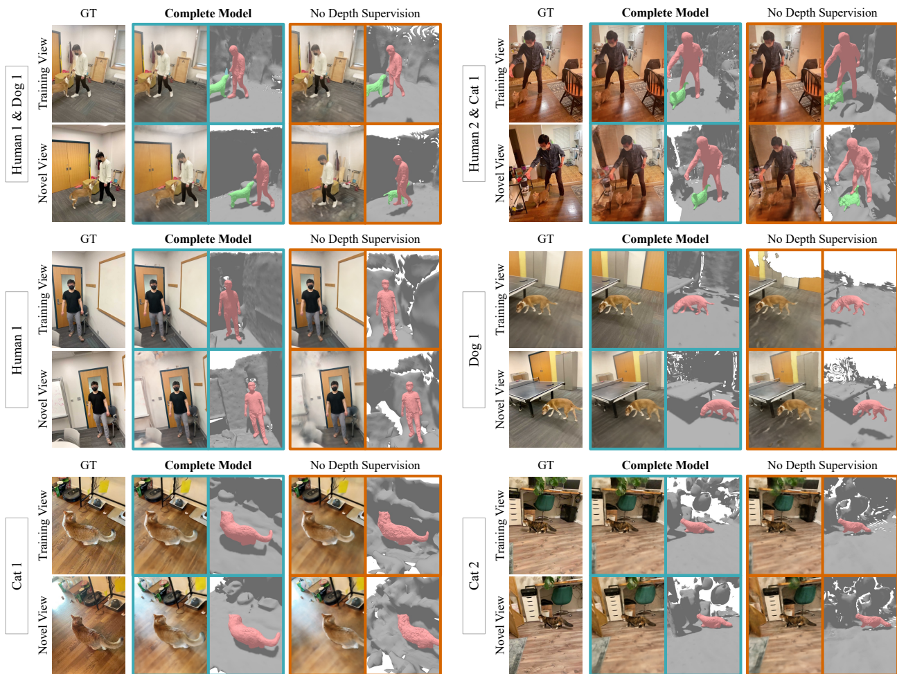
Figure 7: Ablation Study on Depth Supervision. While removing depth supervision from Total-Recon (COMPLETE MODEL) doesn't significantly hamper the training-view RGB renderings, it induces the following failure modes in the novel-view 3D reconstructions. (a) Floating objects : for the HUMAN 1 & DOG 1, DOG 1, HUMAN 1, and CAT 2 sequences, the foreground objects float above the ground, as evidenced by their shadows. (b) Objects that sink into the background : for the HUMAN 2 & CAT 1 sequence, the reconstructed cat is halfway sunk into the ground. (c) Incorrect occlusions : for the HUMAN 1 & DOG 1 sequence, the human is incorrectly occluding the dog. (d) Lower reconstruction quality : for the HUMAN 2 & CAT 1 sequences, we observe that the cat has lower reconstruction quality, and, for all sequences except HUMAN 1 & DOG 1 and CAT 2, we observe that the background object has lower reconstruction quality. Full-length videos can be found at https://andrewsong.github.io/totalrecon/ablation_depth.html .
