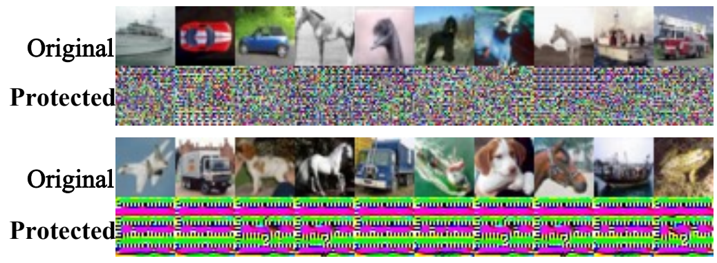
Figure 6: Results of the LIE method and the ITP method. The top group is the result of the LIE method, and the bottom group is the result of the ITP method. Each column represents a different sample.
