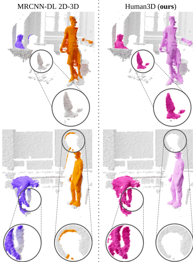
Figure 9: Failure cases of the 2D baseline. The first row shows a typical error of the Mask-RCNN baseline. The sofa occludes most of the human resulting in an incomplete human mask. In addition, the second example shows that small errors at the boundaries in 2D lead to incorrectly predicted 3D points projected far away.
