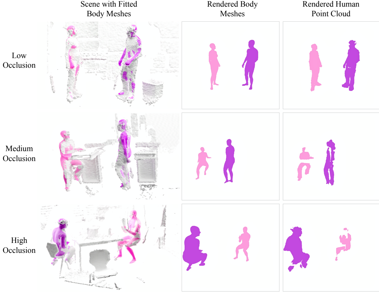
Figure 8: Occlusion Computation. In the first column, SMPL-X human body meshes fitted to humans in the EgoBody dataset are shown. The fitted body meshes for each human ( second column) as well as human masks ( third column) obtained from our manual annotation of the scene point clouds are projected onto an image. Using these rendered images, it is possible to compute an approximation of the occlusion level.
