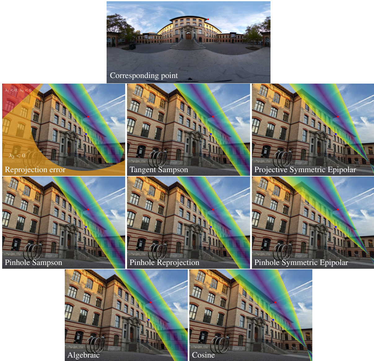
Figure 3. Qualitative comparison of different error functions for a pinhole camera. The thresholds for colormaps were selected to be the error at the point marked by the blue plus. The geometric error is only shown in the region where the 3D point after midpoint triangulation does not correspond to negative depths of bearing vectors (areas where this does not hold for one or both depths are highlighted). Note that level sets for the projection error are slightly curved on the pinhole image because the other camera model is non-linear.
