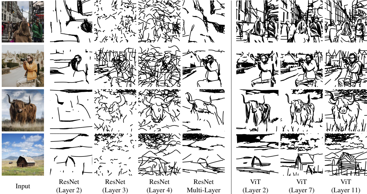
Figure 6. Ablation study on using ResNet-CLIP and ViT-CLIP for guiding the training process. For both variants, we generate the sketches for the entire scene together ( i.e. no scene decomposition is performed) and set the number of strokes to 128. In addition to evaluating ResNet using a single layer for computing \mathcal{L}_{CLIP} , we additionally show results obtained when multiple ResNet layers are used to compute \mathcal{L}_{CLIP} (marked as “ResNet Multi-Layer”). For this variant, we follow CLIPasso [16] as set the layer weights to 0, 0, 1, 1, 0 for layers \ell_1 to \ell_5 , respectively. In addition, we use the output of the fully connected layer and set its weight to 0.1 in the loss computation.
