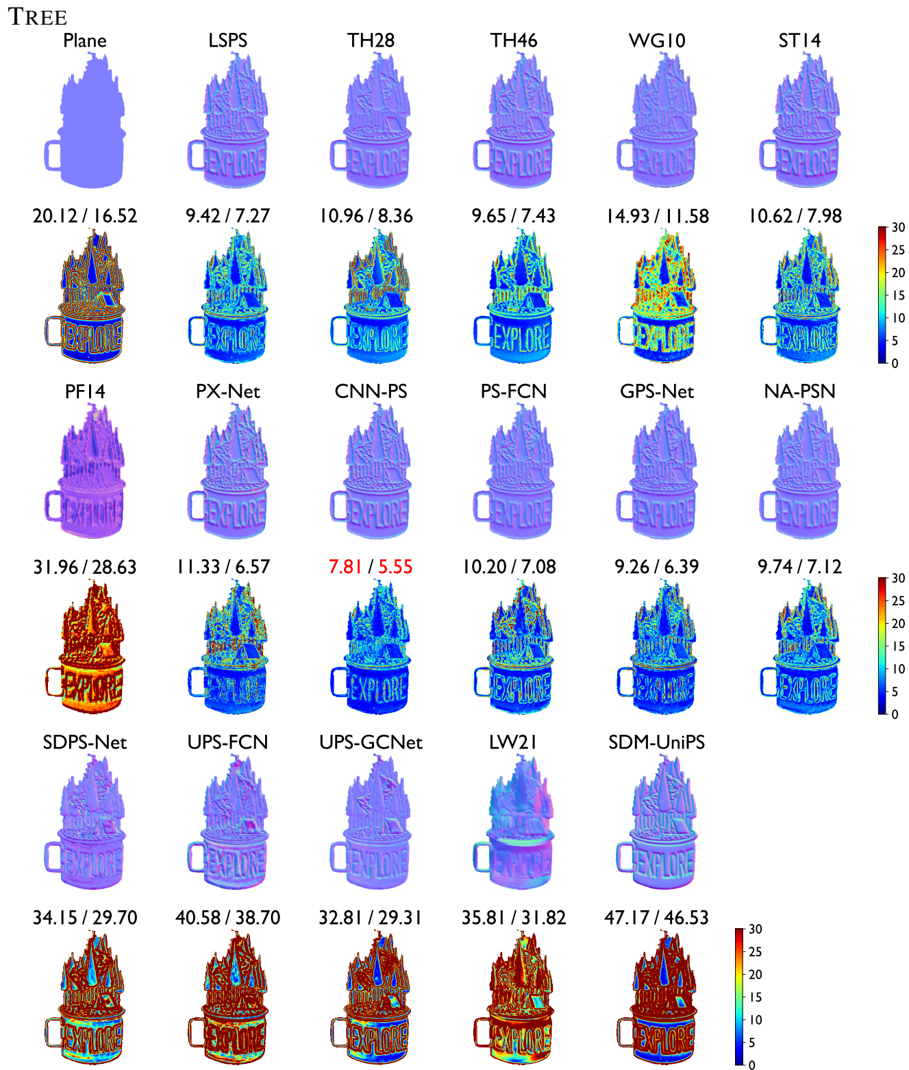
Figure S17: Estimated surface normal maps and angular error maps of TREE.
