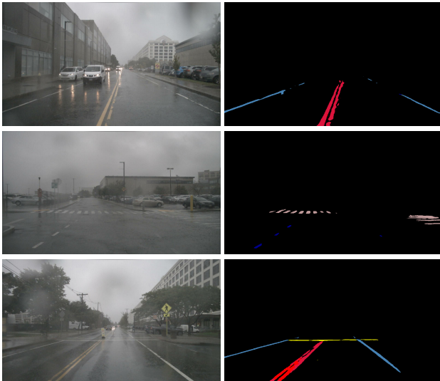
Figure 4: Segmentation results (Right) of real rainy day frames (Left) using the model trained on the artificial ApolloScape Night dataset. The proposed method accurately segments various road lines and markings, including dot lines, solid lines, double yellow lines, stop lines, and crosswalks.
