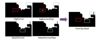
Figure 1: Model ensemble strategy for sky segmentation on VDW dataset. White area represents sky regions. Errors and noises in the rectangles are removed by model ensemble and voting, which improves the quality of the ground truth.
