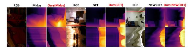
Figure 9: Qualitative results on NYUDV2 [16] dataset. We compare three different single-image depth predictors.
