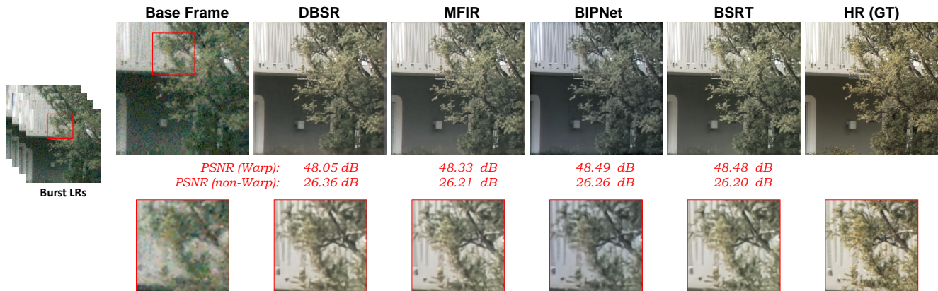
Figure C: Model evaluation of the 0120_0009 image in the BurstSR dataset. ‘Warp’ means that the primary SR prediction is warped with respect to the ground-truth HR image and then used for evaluation, which is evaluation manner in [1]. ‘non-Warp’ means the primary SR prediction is directly used for model evaluation. It is observed that the evaluation with warped results has a very high performance, e.g. , PSNR, while the SR results do not have a very high image quality. Instead, those SR prediction results have a large gap from the ground-truth HR image in terms of the image sharpness and the image color.
