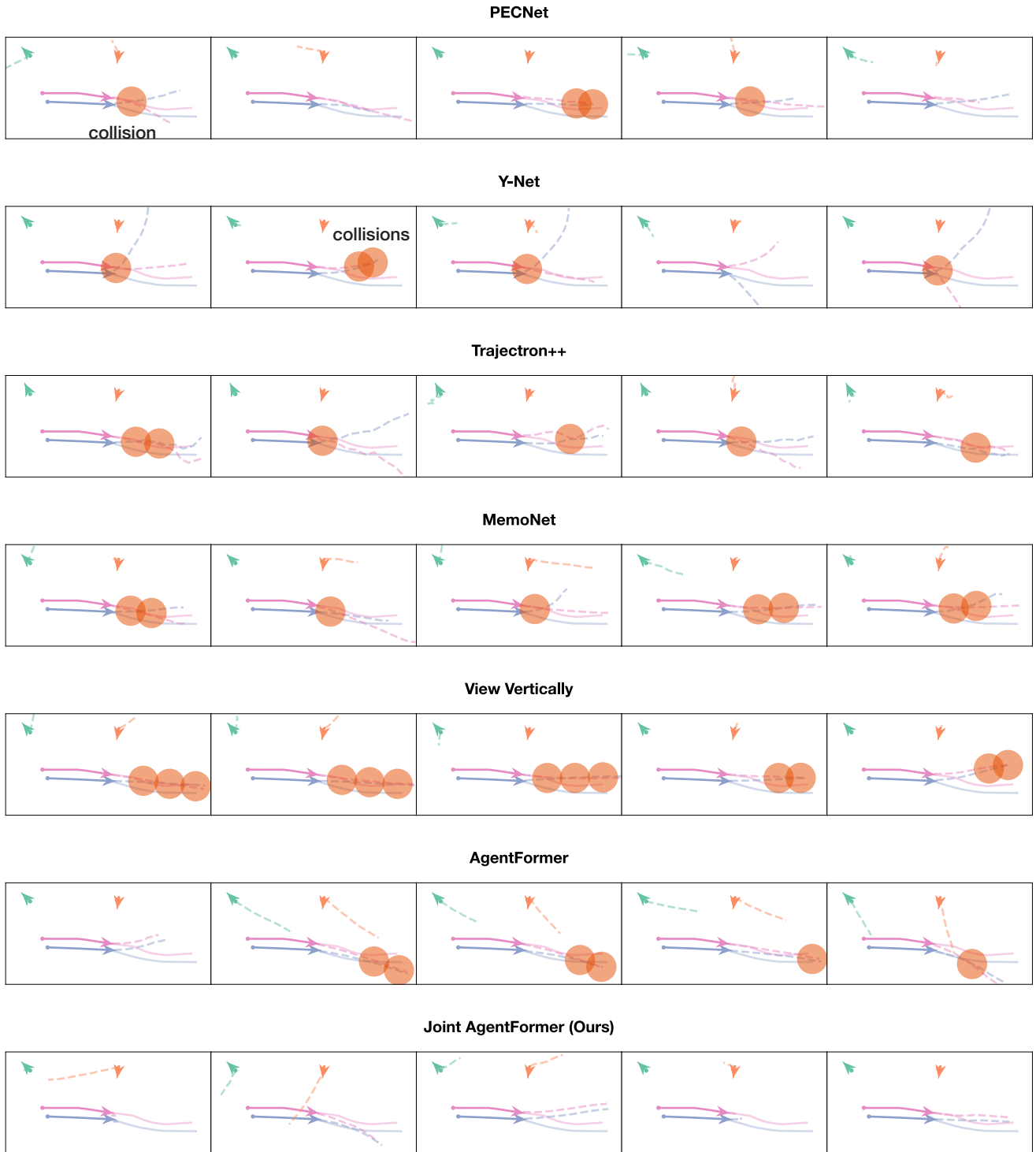
Figure 4: Our method exhibits improved collision-avoidance over baselines. While other methods (first 6 rows), including AgentFormer, predicts trajectories with collisions (denoted by orange circles), our method (last row) predicts trajectories with no collisions.
