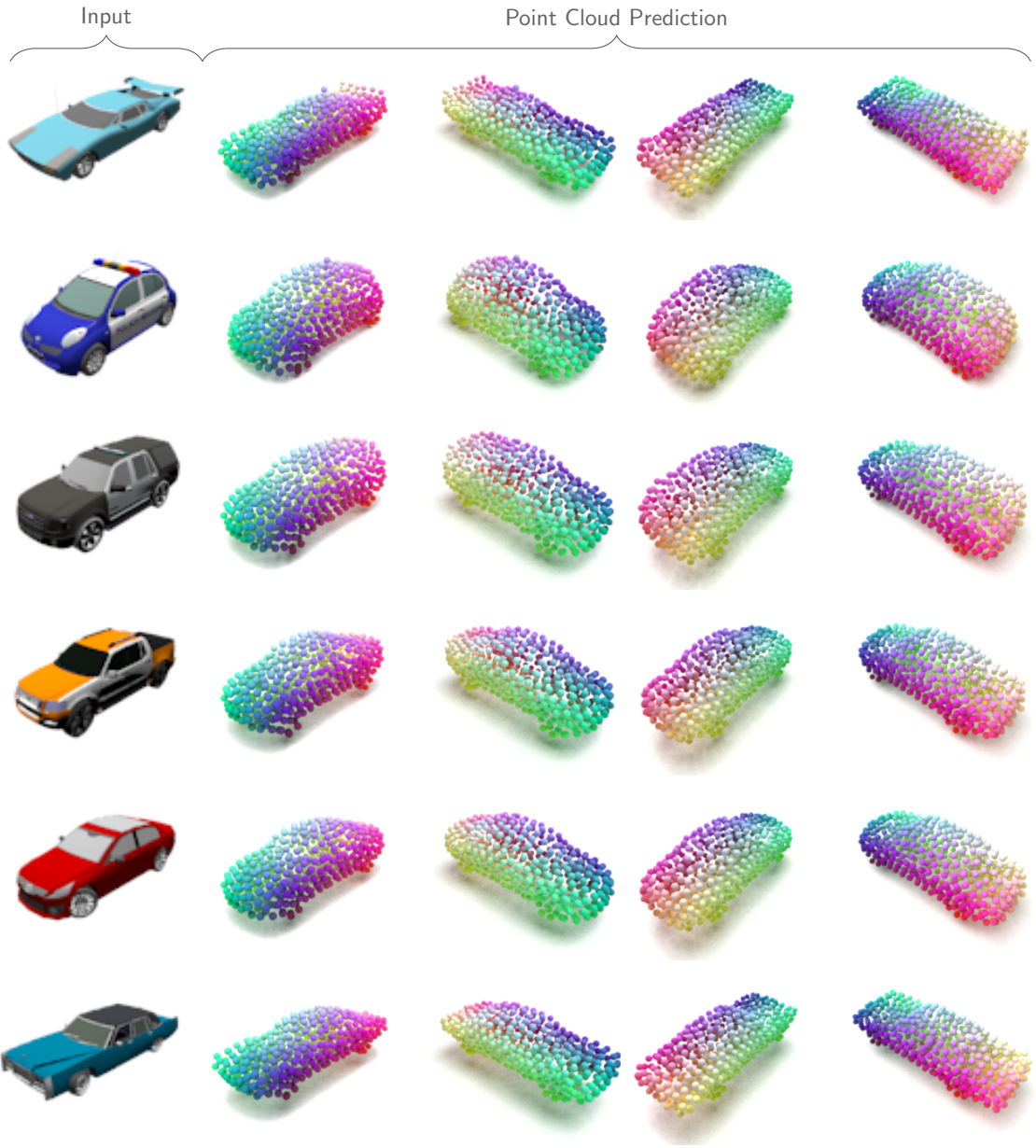
Figure 3: Coherent point cloud prediction. The point color encodes the point identity given by the order of the output tensor that is predicted by the point MLP. It can be seen that these identities behave coherent over multiple instances. This allows the formulation of shared features S . Also, these coherent identities provide correspondences between instances.
