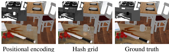
Figure 1: Qualitative comparison of different input encoding shows a hash grid can better model the detailed texture on the floor.
