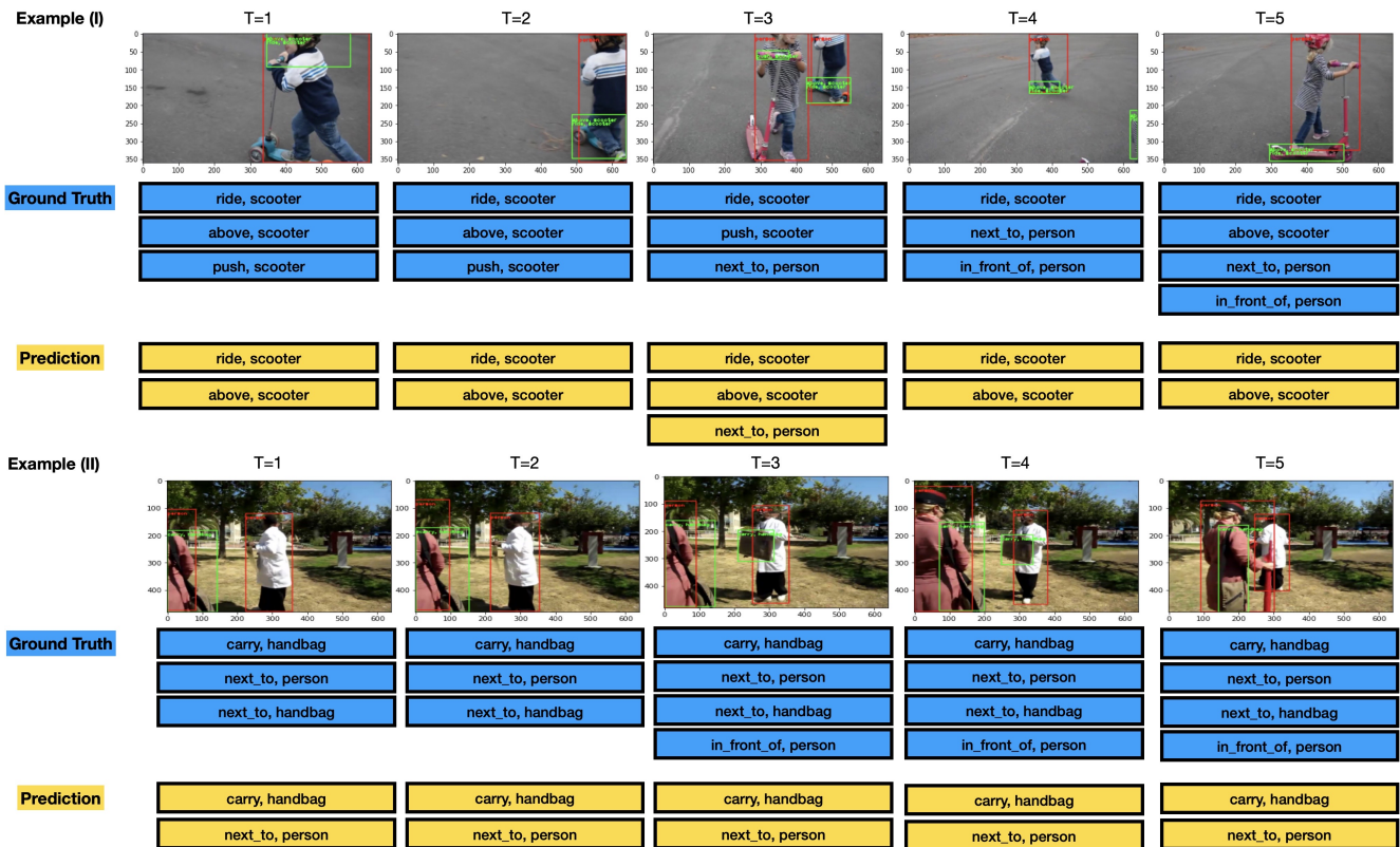
Figure 1: Two examples of video HOI predictions produced by our ACOLP model. Each example consists of five consecutive keyframes. Detected person and objects are highlighted with red bounding boxes and green bounding boxes, respectively. Ground truth and predictions are listed below the frames in the form of “interaction, object”.
