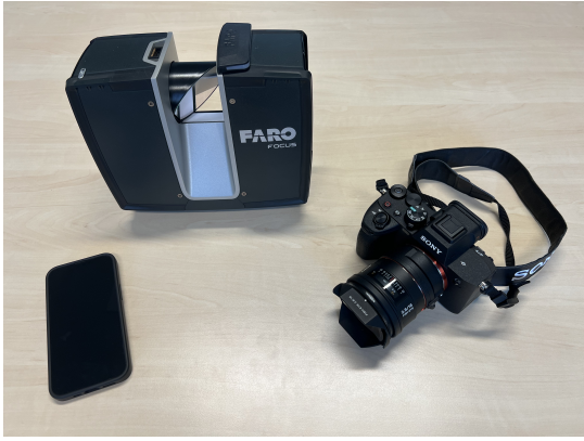
Figure 1: Our hardware setup consists of a Faro Focus Premium laser scanner, Sony Alpha 7 IV DSLR camera, and iPhone 13 Pro with a LiDAR sensor.
