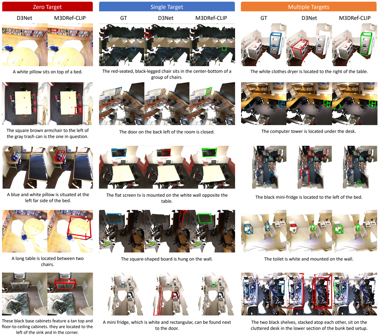
Figure 5: Qualitative results of D3Net [1] versus M3DRef-CLIP on Multi3DRefer using predicted boxes. Blue boxes indicate GT, green boxes are true positives with IoU threshold \tau_{\text{pred}} > 0.5 . Red boxes are false positives.
