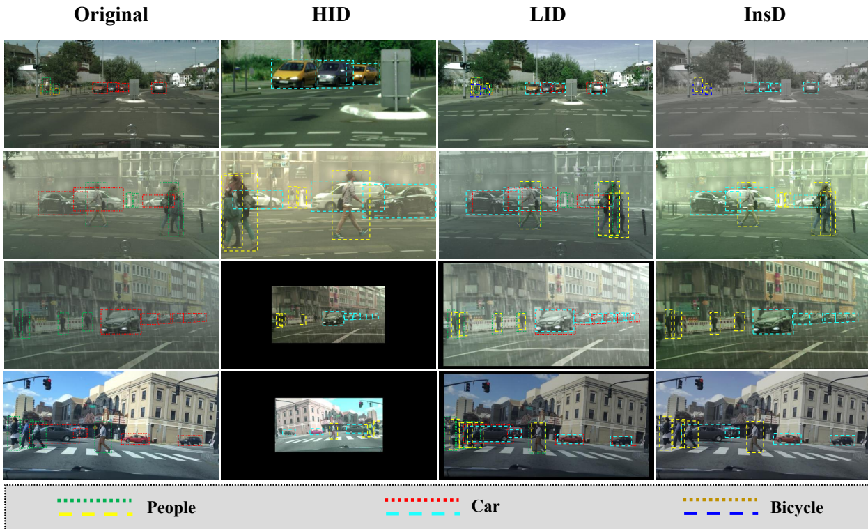
Figure 2. Visualization of several examples of HID, LID and InsD. The dashed rectangles in the images represent the objects under disturbances
