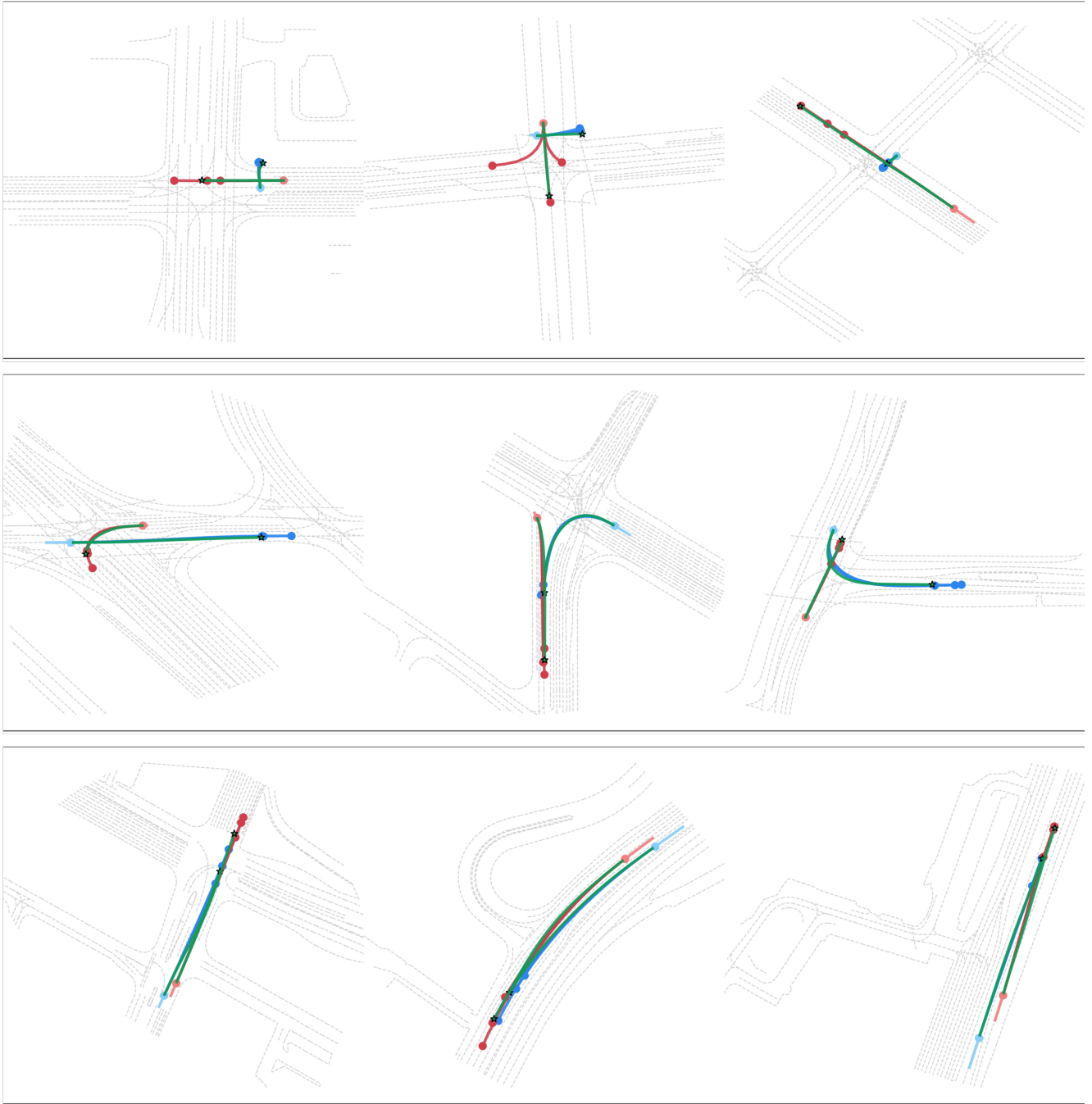
Figure 1. Qualitative results under diverse scenarios on the WOMD interactive validation set. HD map information is shown in light grey. For clarity, we choose K=3 pairs of predicted scene-compliant trajectories shown in red and blue while the corresponding history track is shown in a light color. Ground-truth future trajectories are illustrated in green on the top.
