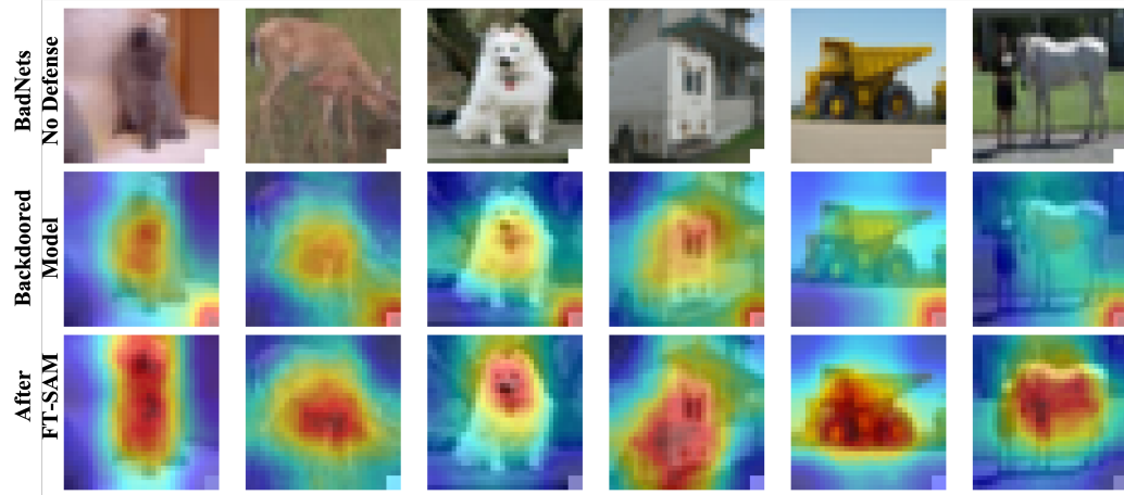
Figure 2. Grad-CAM visualization of regions contributed to model decision under BadNets attack and FT-SAM defense with PreAct-ResNet18 on CIFAR-10.
