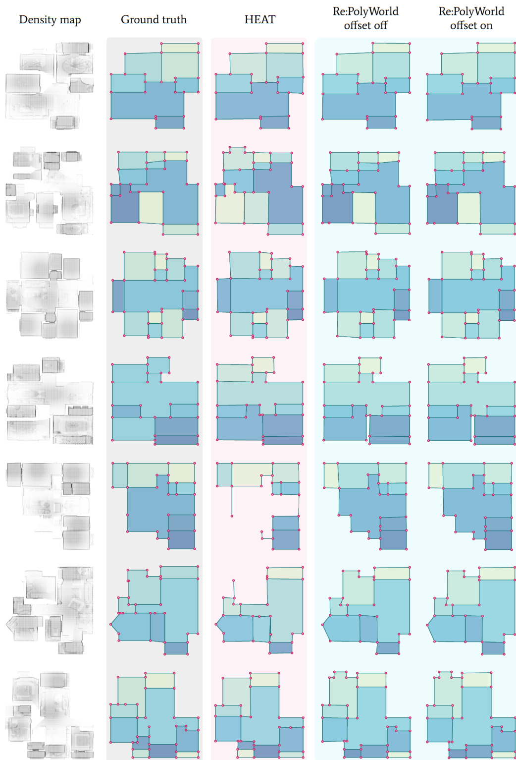
Figure 5. Floorplan reconstruction results on the Structured3D [11] test dataset. Columns from left to right: input density map, ground truth annotations, HEAT [5] results, Re:PolyWorld discarding the positional refinement offset, Re:PolyWorld full method. Please zoom in for better view.
