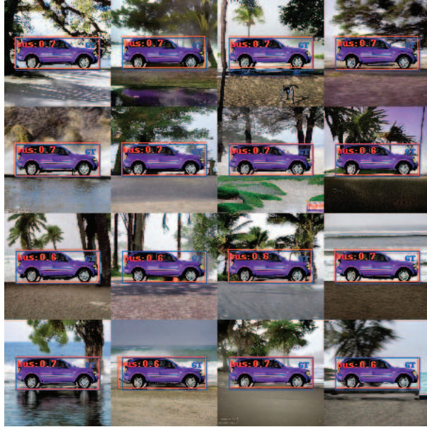
(a) Systematic error into the class bus for the prompt “purple SUV is driving on beach, foggy, idyllic, lush detail”. Here, the image is downscaled by a factor of 4.5 before inputting it into the object detector and the rotation angle is 10^\circ .
