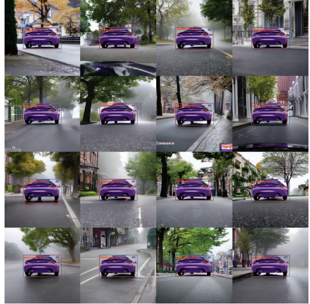
(b) Systematic error into the class suitcase for the prompt “purple coupe car is driving on street, foggy, in the morning, bright, stunning environment, sharp focus”. Here, the image is downscaled by a factor of 2.0 before inputting it into the object detector and the rotation angle is -80^\circ .
