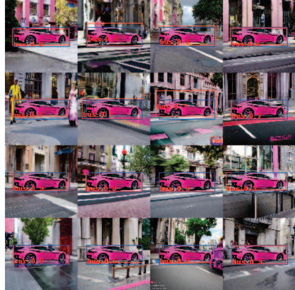
(b) Systematic error into the class bus for the prompt “pink coupe car is driving in city, thundery, in the morning, bright, landscape, HQ”. Here, the image is downscaled by a factor of 5.0 before inputting it into the object detector and the rotation angle is -30^\circ .
