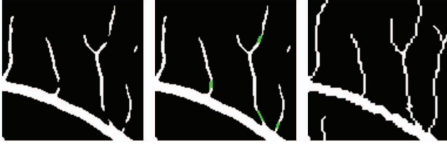
Figure 3. Zoomed images of the Gap Filling procedure: predicted segmentation (left), post-processed segmentation (mid) where filled gaps are drawn green, manually labeled groundtruth (right).
