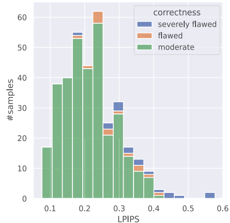
Figure 7. Distribution of the LPIPS error over all Inv3DRealUnwarp samples given by the IllTrTemplate model with a padding of 128 pixels. All samples are classified depending on the severity of the unwarping errors.
