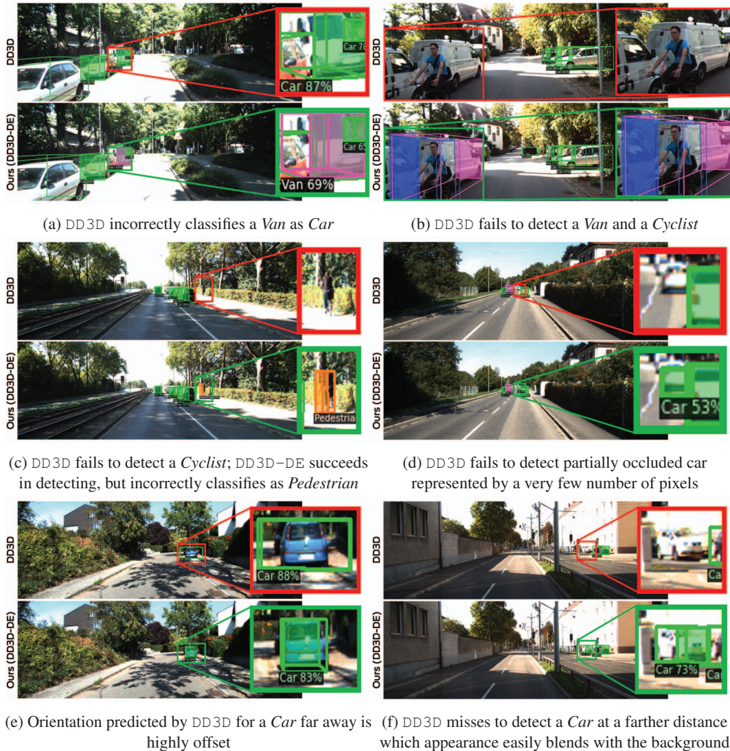
Figure 6: Qualitative analysis of predictions from the baseline DD3D model and our DD3D-DE model. The samples shown here were randomly drawn from the split of the KITTI test split. As shown in the images, DD3D-DE improves the performance over the baseline model on under-represented, and out-of-distribution samples containing objects such as Van , Cyclist , and occluded or far away Car
