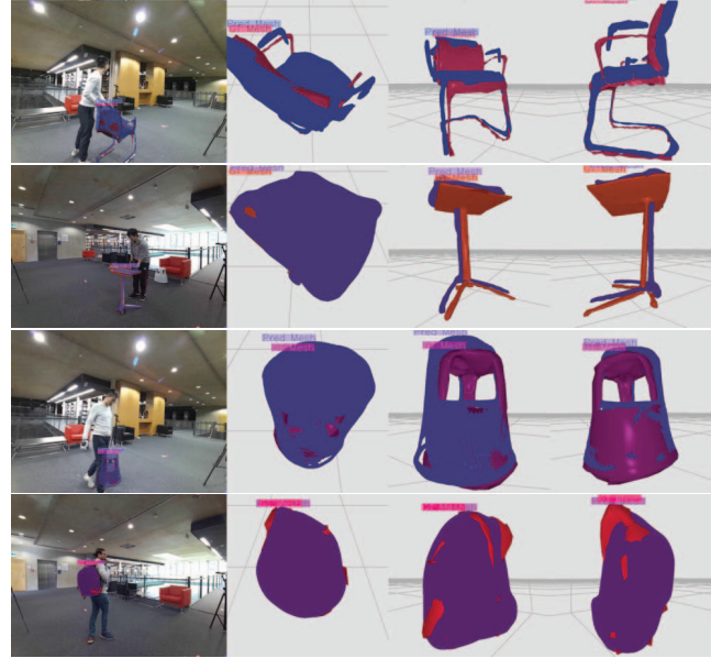
Figure 4. Examples of reconstructed objects on the BEHAVE dataset. We compare the reconstructed (Pred) meshes (blue) to the ground-truth (GT) meshes (red). Input images with overlaid objects are shown on the left and on the right we see the 3D objects projected in three different angles.
