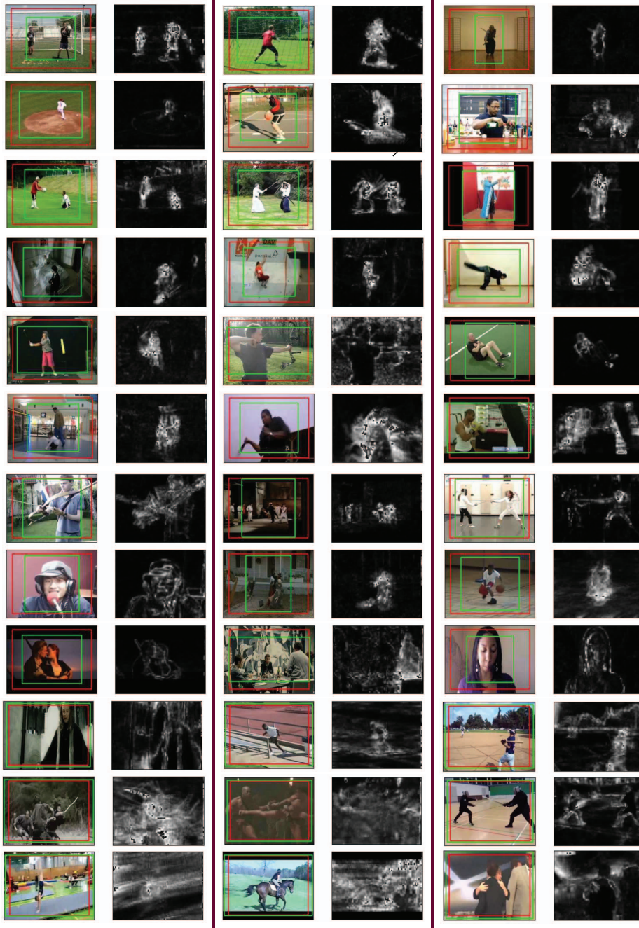
Figure 2. The visualization our proposed adaptive transformation versus center cropping. On the left of each RGB-residual pair of images is the middle frame of a 16-frame video clip, and on the right of each pair is the channel-wise mean of all the 16-frame residual clip. The red and green bounding boxes represent the center crop and our proposed adaptive transformation, respectively.
