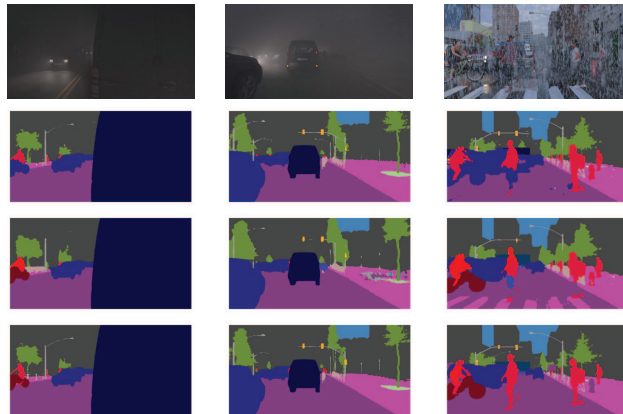
Figure 2: Comparison of predicted segmentation maps. First row illustrate the color images of different adverse weather images. Second to Fourth rows present the baseline model, best individual model and the bias class disagreement ensemble predictions respectively. Each predicted map is codified with the Cityscapes color map [7].
