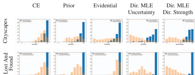
Figure 3: Distribution Separation Plots for in-domain (ID) and out-of-domain (OOD) dataset. Dirichlet MLE demonstrates superior separation for both uncertainty and Dirichlet strength.
