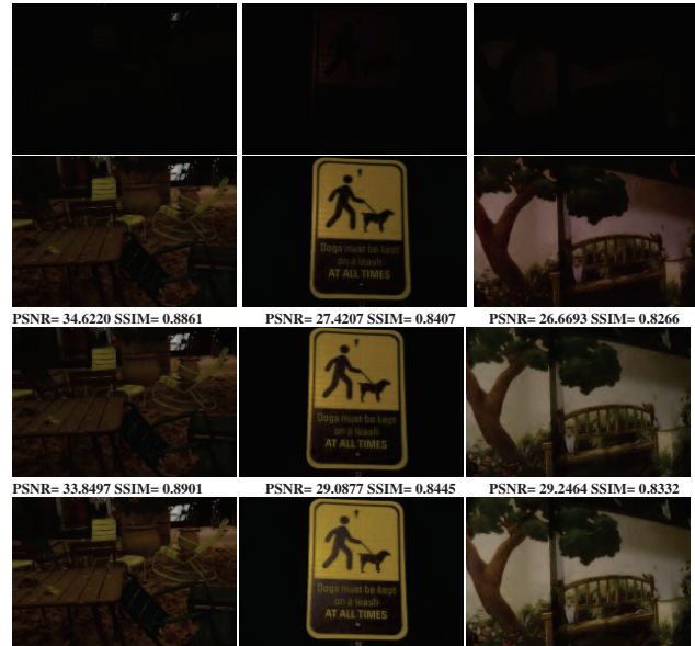
Figure 8: 1 st row represents input images (SID Dataset [3]), 2 nd row represents results of authors in [18], 3 rd row represents results of proposed method LightNet, and 4 th row represents the ground-truth images. We infer, the proposed LightNet restores color, contrast, and luminance consistently.
