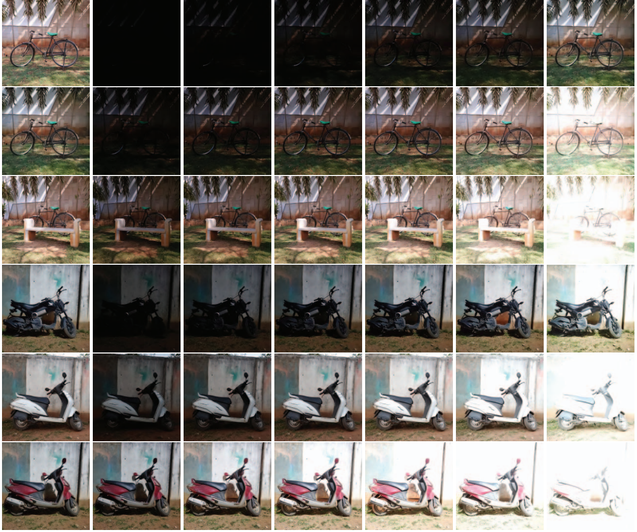
Figure 5: Images captured in low-light conditions, 1 st column shows ground-truth image (captured in auto settings), 2 nd column shows images capture with ISO50 , 3 rd column shows images captured with ISO100 , 4 th column shows images capture with ISO200 , 5 th column shows images captured with ISO400 , 6 th column shows images captured with ISO800 , 7 th column shows images captured with ISO3200 . Exposure is fixed across the rows (1 st row : 1/24000s , 2 nd row : 1/4000s , 3 rd row : 1/2000s , 4 th row : 1/180s , 5 th row : 1/20s , 6 th row : 1/2s )
