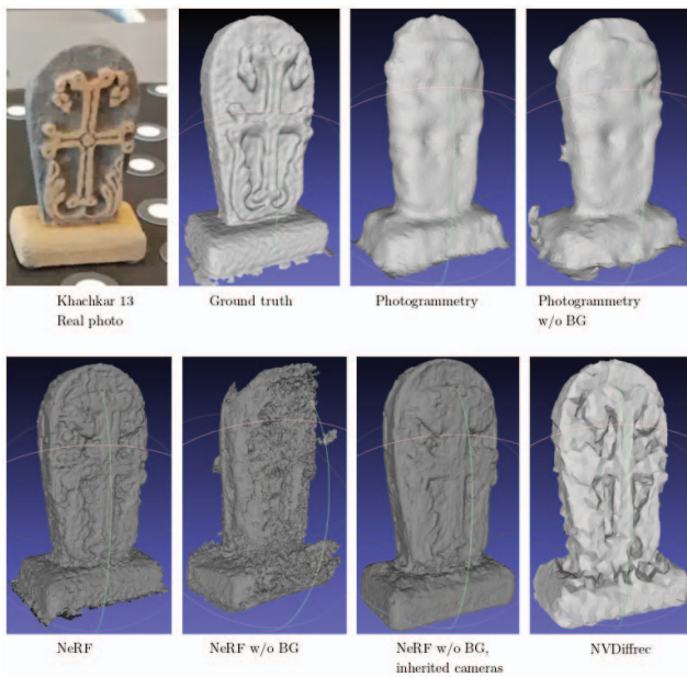
Figure 2. Khachkar 13 reconstructions. The minimum for total CD is Photogramm. w/o BG. The minimum for forward is Photogrammetry w/o BG and for backward is NeRF w/o BG, inherited cams.
