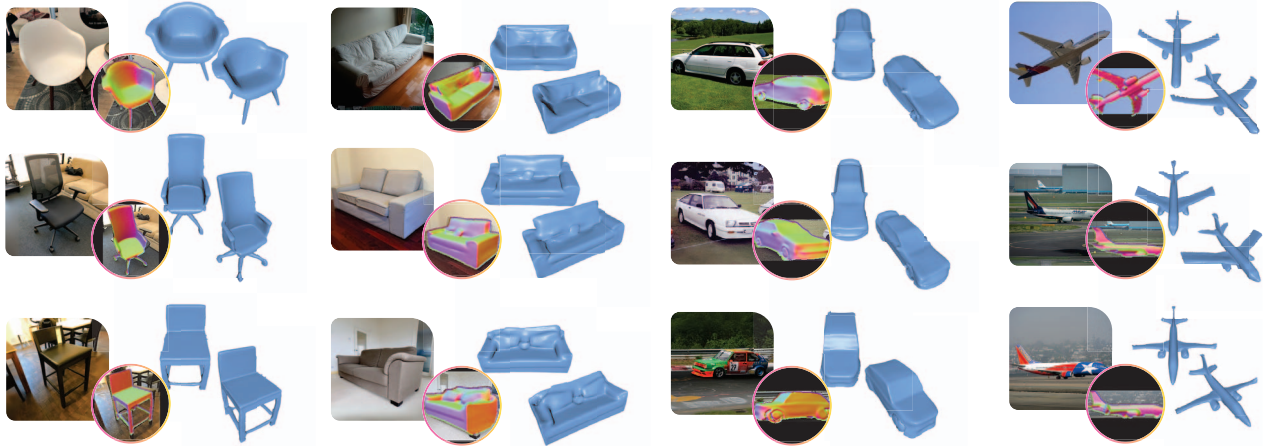
Figure 1. We present SDFit, a novel framework that recovers an object’s 3D pose and shape from a single image. To this end, SDFit uses a learned, category-level, morphable SDF (mSDF) shape model, namely DIT [77], and fits this to images in a render-and-compare (a.k.a. analysis-by-synthesis) fashion. SDFit is robust to occlusions and uncommon poses, and requires no retraining for in-the-wild images. For visualizing the fitted mSDF overlaid on the input image, we show the mSDF’s normals with color coding. Q Zoom in for details.
