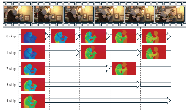
Figure 3. Optical flow with different skip levels. RelayFlow-4K provides flows for adjacent frames (0 skips) and cross-frame flows up to 4 skips, which are uncommon in standard datasets.
