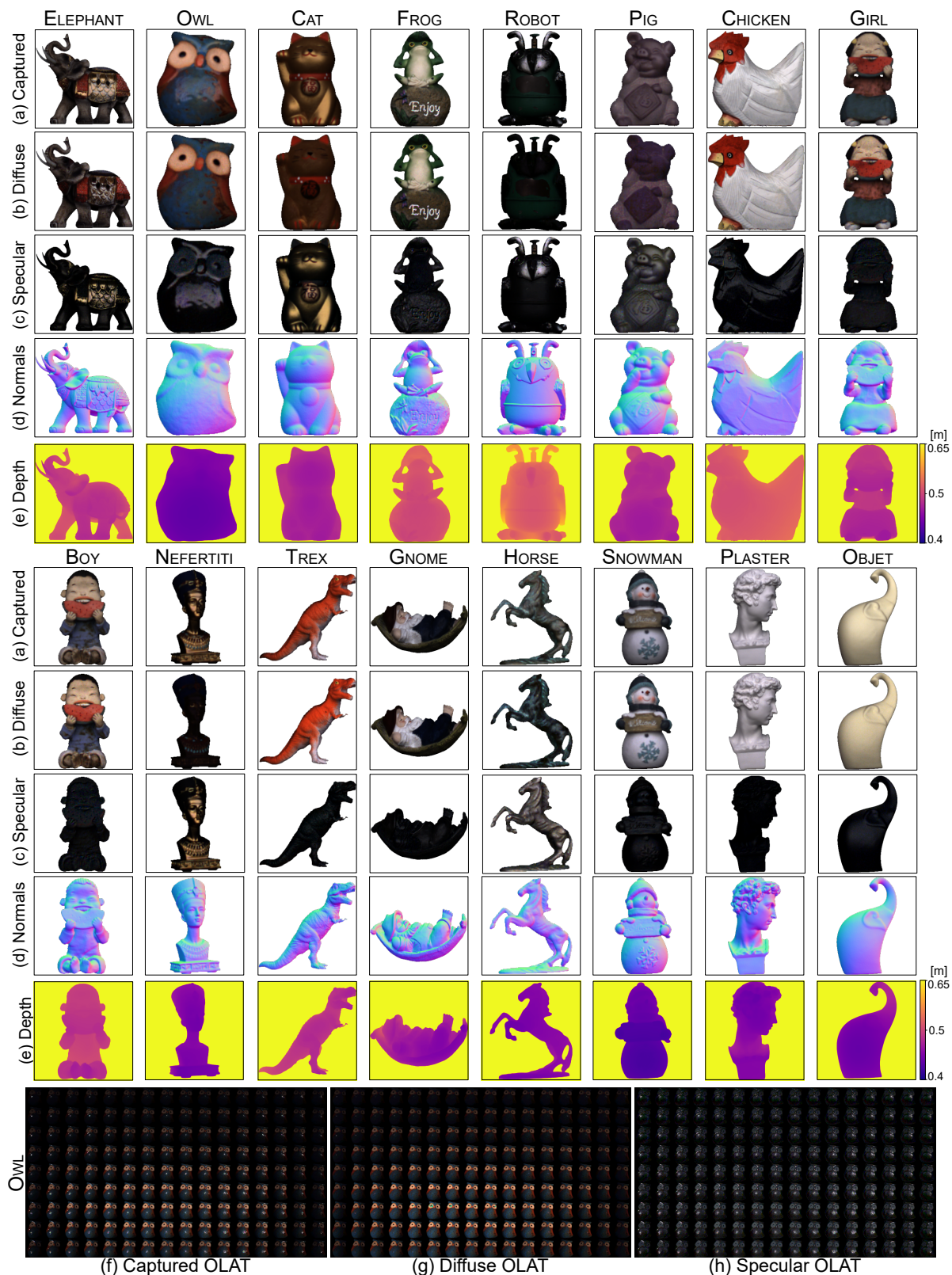
Figure 2. Display Inverse Rendering Dataset. We introduce the first display inverse rendering dataset. We obtain (a) combined, (b) diffuse, and (c) specular stereo images captured under (f–h) OLAT patterns. We provide ground-truth (d) normal maps and (e) depth maps.
