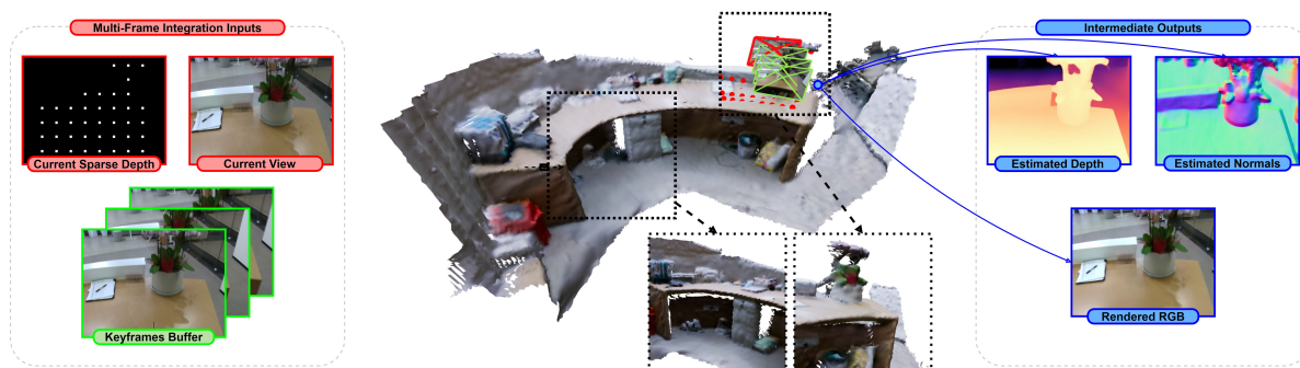
Figure 1. Overview of our ToF-Splatting method. Our method combines sparse ToF depth, multi-view geometry from a buffer of keyframes, and monocular cues (left) to perform into a unique end-to-end dense SLAM framework enabled by a Gaussian Splatting.
